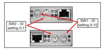
Ex. The 0-7 switch is set to 2, the 0-15 switch is set to 6. This sets the base address to 38 (2\*16=32, +6=38). So Slot 0 ID = 38, Slot 1 ID = 39, Slot 2 ID = 40, Slot 3 ID = 41, etc... up to Slot 9 ID = 47.
